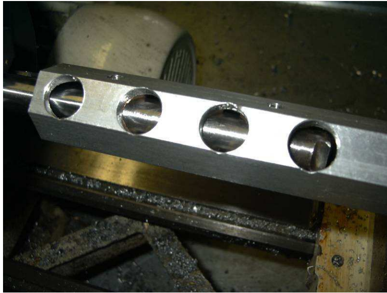
Using the D-bit reamer to remove burrs.
