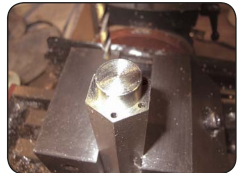
Drilling screw holes in Backplate
