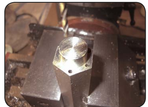
Drilling screw holes in Backplate
