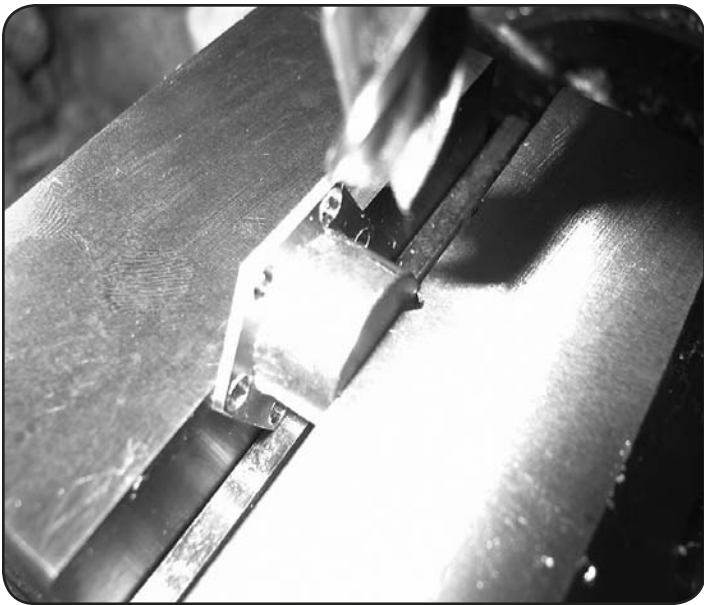
Milling clearance for Piston
